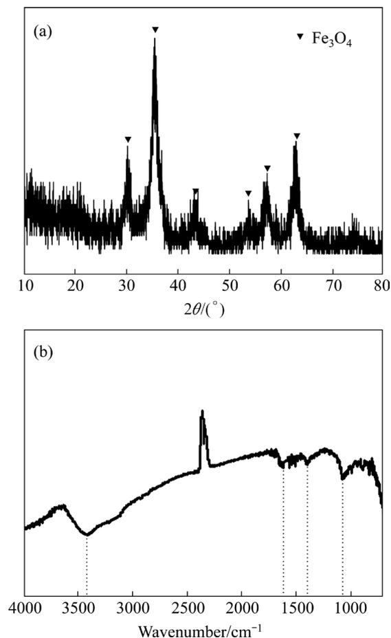
**Fig. 3** XRD pattern (a) and FT-IR spectra (b) of Fe<sub>3</sub>O<sub>4</sub>@chitosan-3
