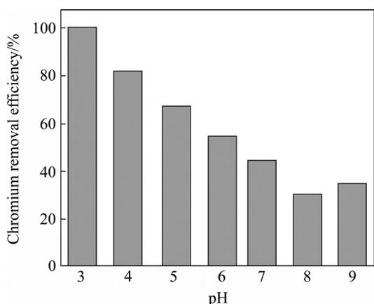
Fig. 5 Effect of pH on chromium removal efficiency
