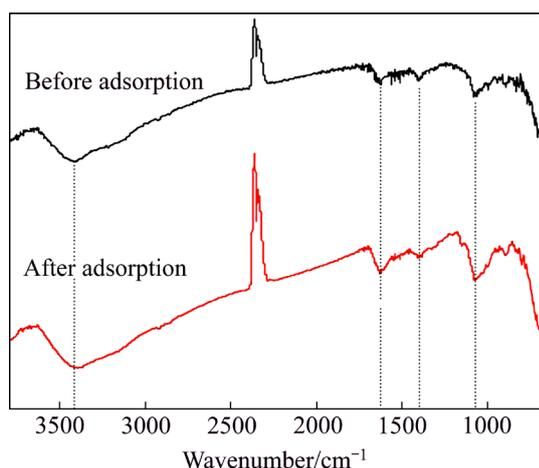
Fig. 7 FT-IR spectra of  $\text{Fe}_3\text{O}_4$ @chitosan-3 before and after chromium adsorption
