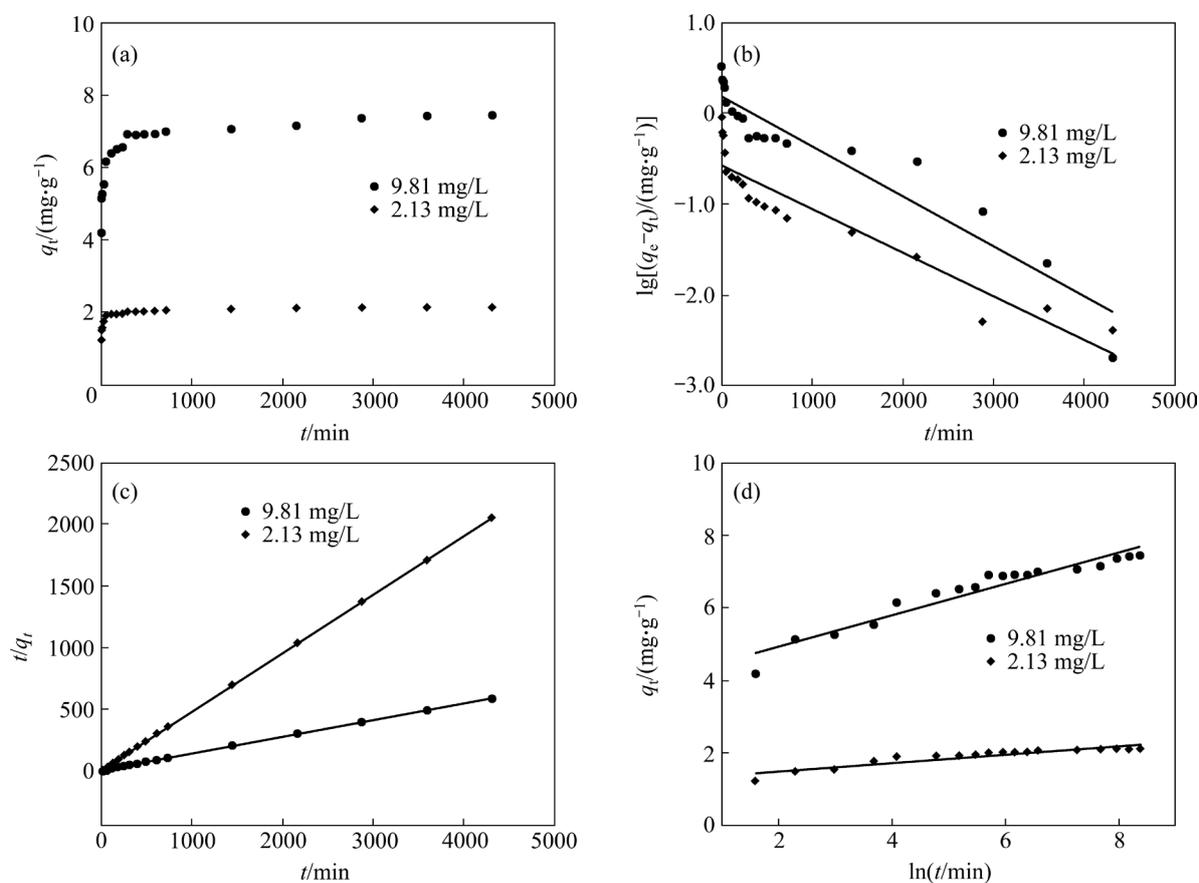
Fig. 6 Effect of reaction time on Cr(VI) adsorption: (a) Kinetics modeling of Cr(VI) adsorption; (b) Pseudo-first-order kinetic plots; (c) Pseudo-second-order kinetic plots; (d) Elovich model plots ( $t$  is the reaction time;  $q_e$  (mg/g) and  $q_t$  (mg/g) are the amounts of adsorbed Cr(VI) at equilibrium and at any reaction time  $t$ )
