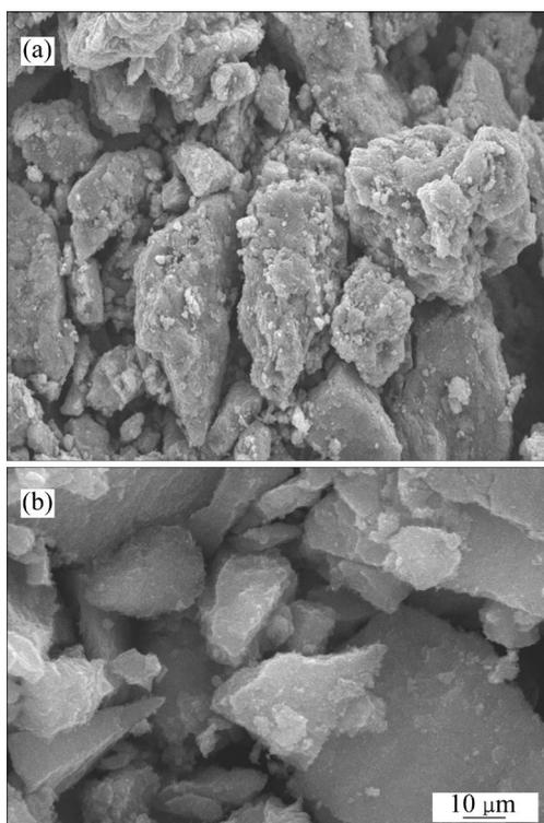
**Fig. 2** SEM images of Fe<sub>3</sub>O<sub>4</sub>@chitosan-3 (a) and Fe<sub>3</sub>O<sub>4</sub>(b)
