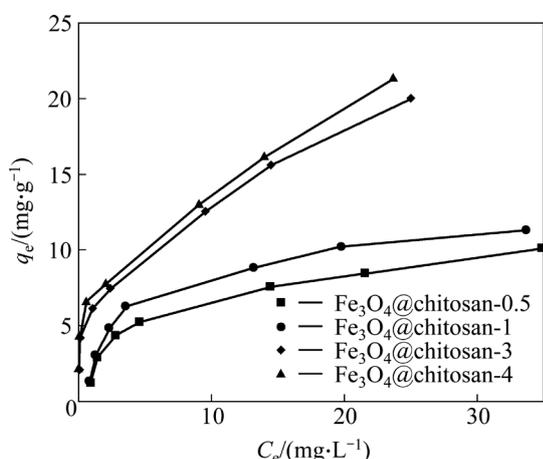
**Fig. 1** Adsorption isotherms of Cr(VI) on Fe<sub>3</sub>O<sub>4</sub>@chitosan composites with various of mass ration of Fe<sub>3</sub>O<sub>4</sub> to chitosan
